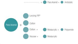
Aramid fibres are high performance fibres with excellent heat resistance and a high tenacity to elongation ratio at breaking point.
